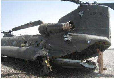
A15-103 in situ, emphasizing failed landing gear (Photo by C Kerr)
